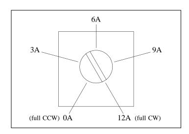
The setting should be adjusted to a comfortable level above the running current expected for the actuator <u>and</u> its load. When the motor current exceeds the **Trip Setting**, the motor is turned off, the yellow LED is turned on, and the form-C contact switches.
