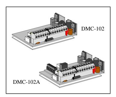
The DMC-102 has a fixed current trip threshold of 12A. The DMC-102A has an adjustable current trip feature (adjustable from 0 to 12A) that is useful for limiting torque to the load or to protect motors that have less than 12A locked rotor current. The DMC-102A also has a yellow LED trip indicator and a set of form-C contacts that can be used to power external alarms or lights.
