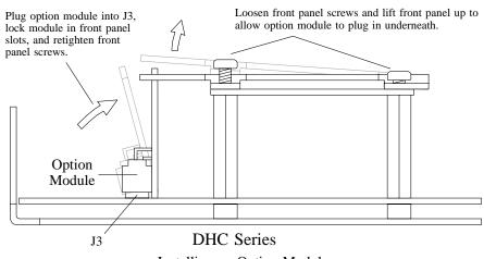
Installing an Option Module
