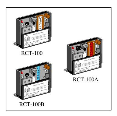
The unit is available in versions for various power sources (50/60 Hz) and has a minimum motor load requirement due to its trickle current: RCT-100 (117VAC  $\pm 10\%$ , 0.2A minimum load), RCT-100A (234VAC  $\pm 10\%$ , 0.1A minimum load), and RCT-100B (24VAC  $\pm 10\%$ , 1A minimum load). The encapsulated enclosure with wrap around bracket makes it rugged and easy to mount to the mid-section of an actuator using the two mounting legs located on the back side of the unit.
